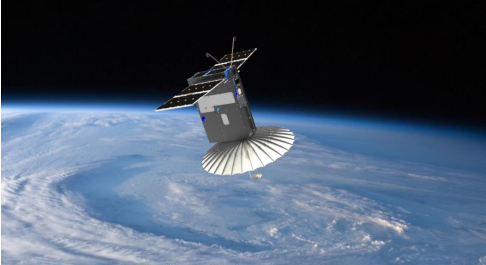
RainCube's deployable antenna / Image: Tyvak-Jonathan Sauder-NASA-JPL Caltech via Space.com.
